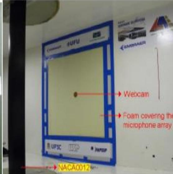
External and Internal View of the Wind Tunnel Antenna
